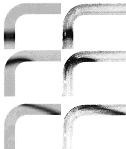
Figure 6. Simulation (left column) and photobleached-fluorescence visualization (right column) of an analyte band traveling around a constant radius corner. In both cases the channel is 250 \mu\text{m} wide. In the experiments, the channels were \sim 40 \mu\text{m} deep. The transport ratio, t_{\text{turn}} was \sim 500 .
