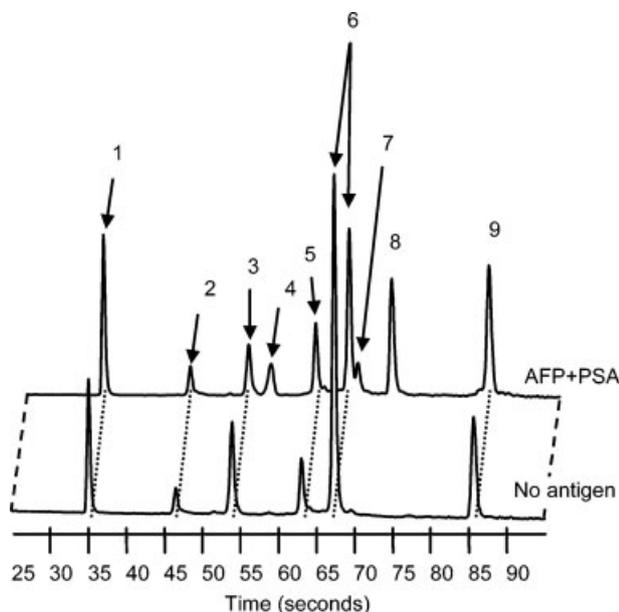
**Figure 2.** Electropherograms from affinity-based MCE show simultaneous detection of PSA and AFP using mobility-modified mAbs. The PSA mAb was conjugated to 245-bp DNA, while the mAb to AFP was conjugated to 626-bp DNA. Reprinted from [44], with permission.
