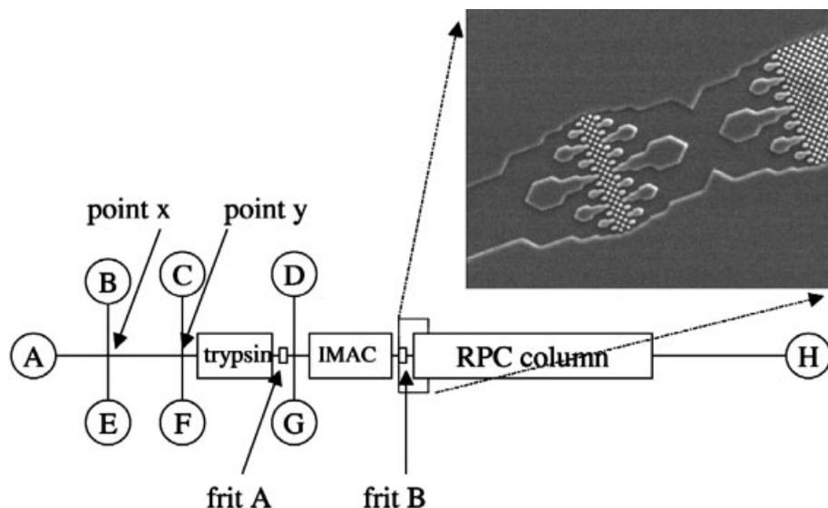
**Figure 3.** Single chip integration of trypsin digestion, copper (II)-immobilized metal affinity chromatography (Cu(II)-IMAC) selection of histidine-containing peptides, and RP CEC of selected peptides. Reprinted from [62, with permission.
