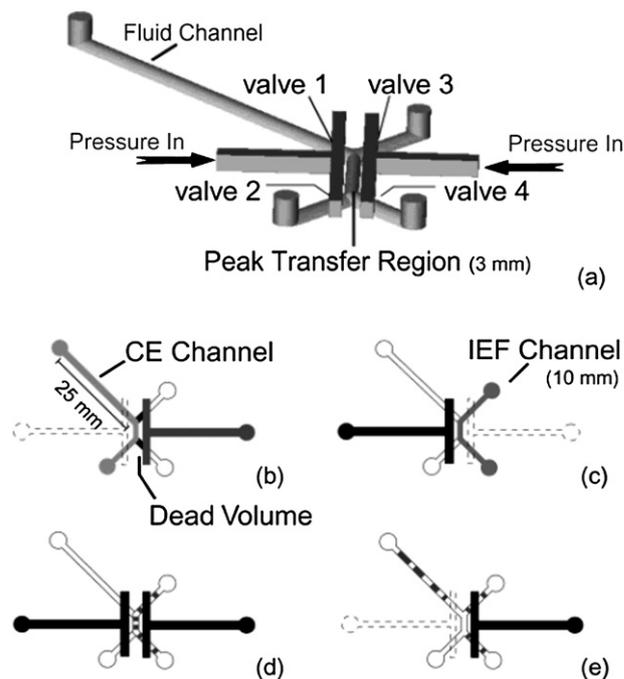
**Fig. 4** The double layer PDMS channel is actively engaged through four distinct stages of separation: (a) perspective view; (b) CE buffer loading; (c) IEF ampholyte mixture loading; (d) isolation of target proteins by closing all valve sets; (e) further separation of isolated proteins. Reprinted with permission from Wang *et al.*<sup>41</sup> Copyright 2004 American Chemical Society.
