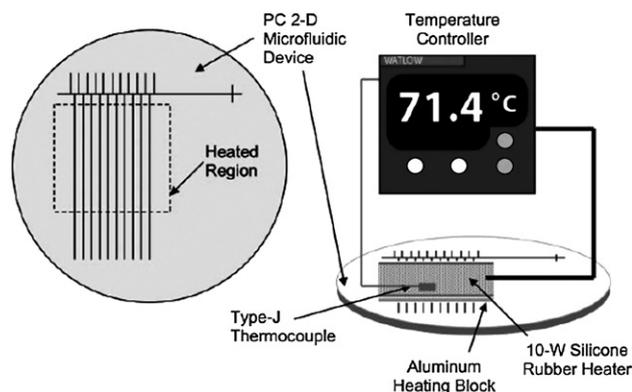
**Fig. 7** Illustration of the temporal temperature control set-up for on-chip denaturing gradient-based two-dimensional gene mutation scanning from Buch *et al.*<sup>115</sup> Reproduced by permission of the Royal Society of Chemistry.
